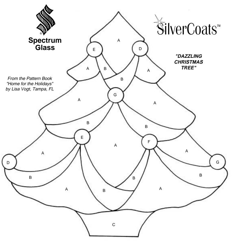
**Note:** Project can be displayed in a fan lamp holder. Complete as shown for a sparkling reflective tree. Substitute transparant nuggets (D, E, F, G) for a tree with glowing lights when used as a fan lamp.
